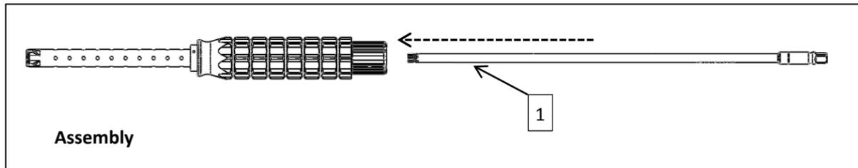
**Glenoid Augmented Reamer (1230-5205) - Disassembly / Assembly**
